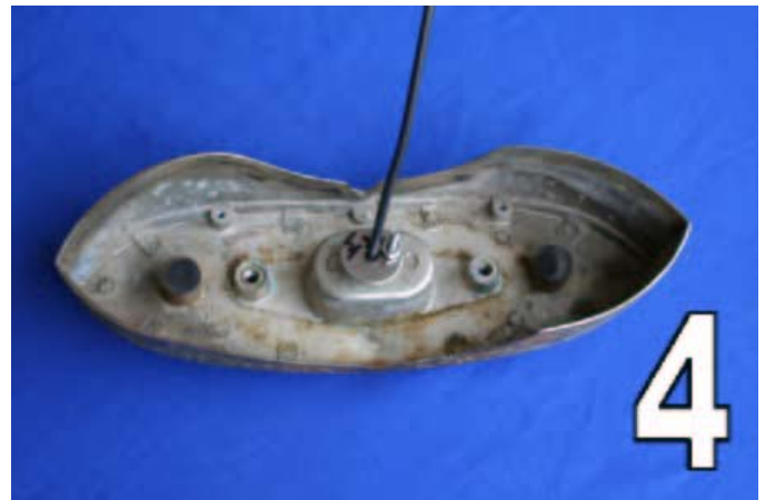
Tighten nut after LED is squared in the housing.
