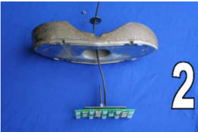
Pass the LED wire through the taillight and brackets as shown.
